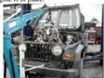
Use the 1/2" bolts and nylon nuts to secure the engine to the frame. Bolt the steering pillow block assembly to the mount. Take a quick look around the engine and steering to make sure there are no clearance issues. You should have just enough room to fit your hand between the engine and firewall/frame.
