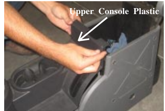
Figure 10: Removing Upper Console
