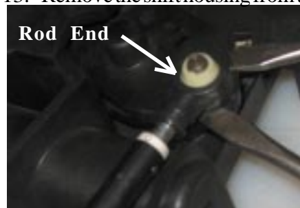
Figure 12: Rod End Removal
