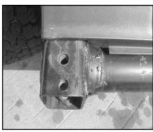
Remove old bumper from vehicle frame using #55 Torx bit. Save the Torx bit bolts, they will be used to mount your new bumper. Remove the plastic sway bar cover using 3/8" wrench. For 97 and newer TJ Wranglers remove the front bolt of each sway bar mount using 15mm wrench. See photos 1&2. Arrow points to the OEM sway bar cover that must be removed. Sway bar cover is different on 1988-1995 Jeeps.
