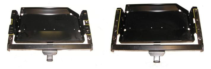
Shown above is the Jeep-sourced hitch installed with our gas tank skid plate above the hitch on the left and below it on the right.
